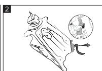
Disconnect the fuel pump cover cable and the fuel connector as indicated in the
