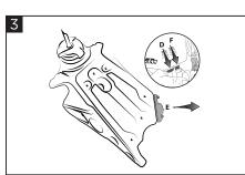
Remove the pump (E) and the fasteners (D/F) from the original tank.
