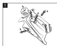
Empty any remaining fuel from original fuel tank. Remove the seat, side panels and radiator scoops. Remove the screws (B) that fixing seat, radiator scoops and tank (G). Syuotare completamente la benzina dal
