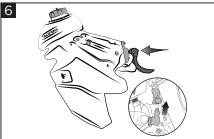
Reconnect the fuel pump power cable and the fuel connector. Assemble the radiator scoops, side panels and seat.
